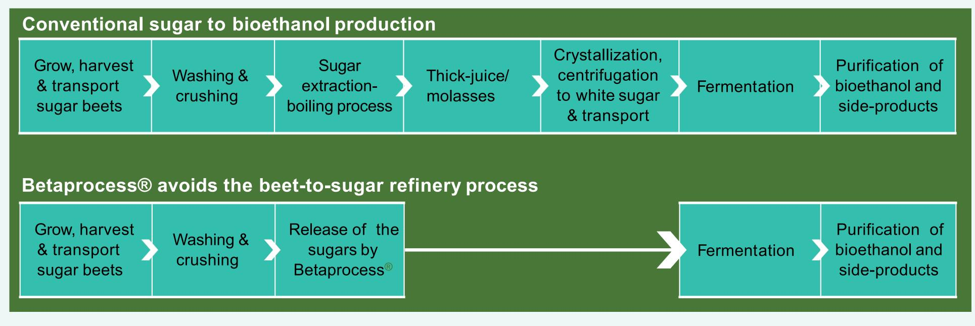
Main advantage of the new technology is that it avoids the beet-to-sugar refinery process. The beet-to-ethanol process is thereby reduced by two production steps.
